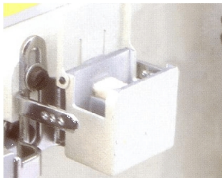
showing the upper HR-device for lubricating the needle threads (used optional)
