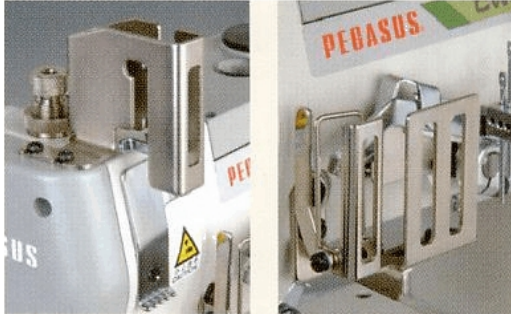
left and right picture: traditional thread take-up with finger deflector
