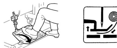
**[AUTO]** Every time sewing is completed, the tape (elastic) is inserted automatically.
