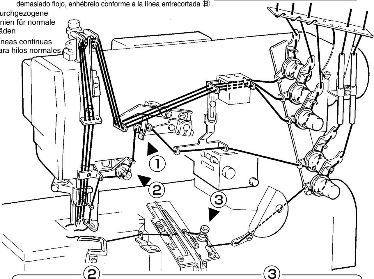
**D**: Lines discontinuous **D** apply to very elastic threads.
