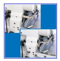
High axis is used for knitted fabric and Jeans machine. Low axis is used for woven fabric to reduce puckering.
