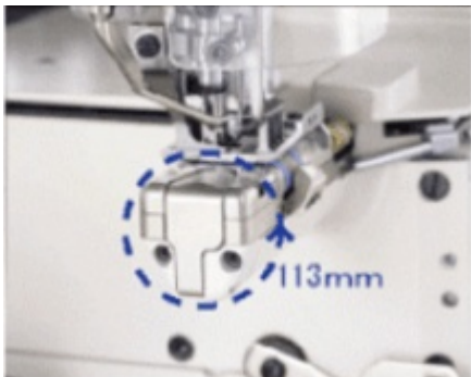
The very small arm of WT169 with a circumference of tiny 113 mm.
