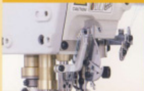
Cam : Down position (Soft seam)
