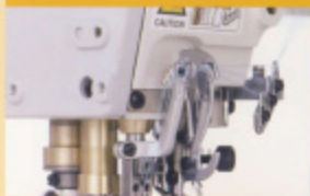
Cam : Upper position (Tight seam)
