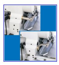
High axis is used for knitted fabric and Jeans machine. Low axis is used for woven fabric to reduce puckering.
