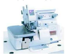
This new developed subclass is especially made for the application of butt seaming and offers a wide seam of 6 mm, which has opened a seam width of 12 mm.
