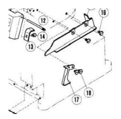
Item (17) with parts no 211109 is correct and item (23) with parts no 211109 has to be changed to parts no. 211311 in case of E22L and 21174 in case of E32L
