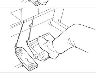
4. Complete sewing. In order to cut thread chain smoothly, stop feeding a fabric when the thread chain is sucked into the suction inlet  ${\bf 1}$ . (See the illustrations below).
