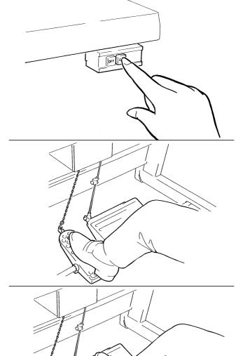
3. Start sewing by pressing the machine treadle.
