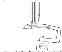
The point of the left needle has reached the bottom end of the looper blade.
