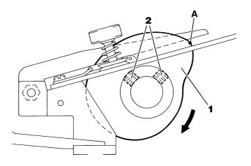
Position of the point of the left needle when the looper thread is released from point A on looper thread take-up 1.
