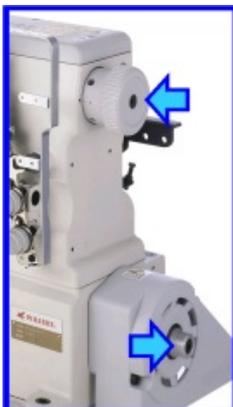
Hand wheel is fully enclosed like on W2600, avoiding any winding of threads round the shaft
