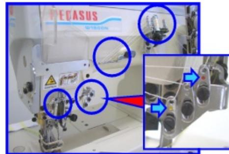
By marking the thread guides with a colour code, each thread has it's own colour, to prevent wrong threading by the operator.
